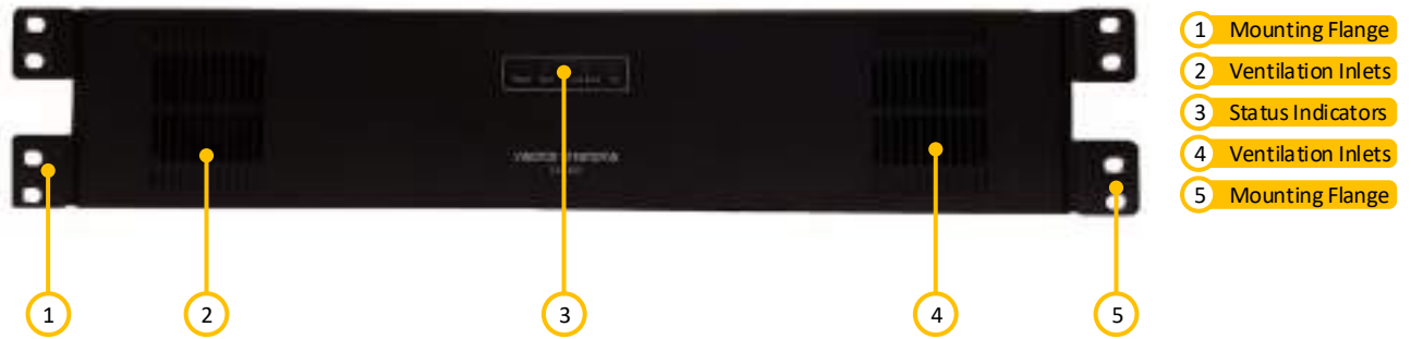
Figure 36 EA amplifier schematic front panel
